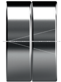
Outer raceway markings for paired bearings
